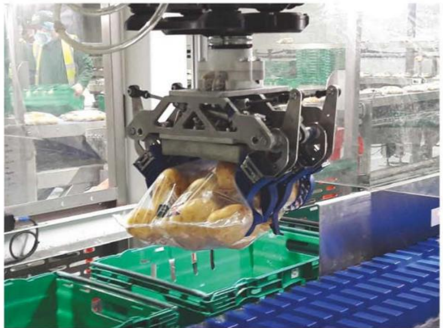
Brillopak's innovative Glove revolutionises how heavy fresh foods, including potatoes, melons, meat joints and netted produce is packed into retail crates and trays using automation.
